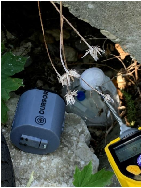
Fig. 4: Measure by the Sniffer and the PID controller of VOC presence from a mixture of cadaver specific VOCs in a hole inside the rubble.
