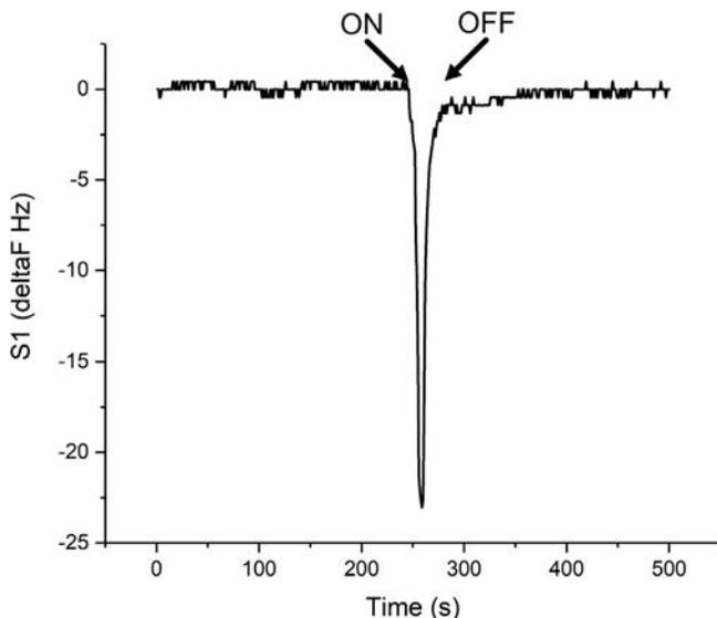
**Fig. 12** Raw data response of an OBP-QMB sensor to cocaine-HCl vapor. A saturated vapor headspace was aspirated across the sensor array and the frequency change of each sensor was recorded. A decrease in frequency is observed as the mass of the QMB increased due to the loading of the adsorbed analyte, and this is reversible when clean air is applied to the sensor.
